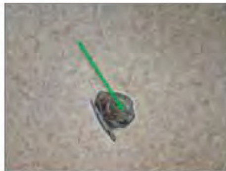
✓ 10042:1+12018:1. Mörkbrunt lim under dold linoleum. Ej asbest.
